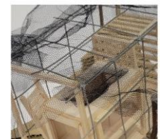
Grid Made of steel, acting as a structural frame, and accommodates spaces, giving translucency and a lightweight look.
