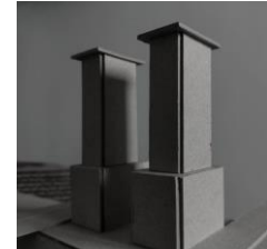
WIND TOWERS provide ventilation by distributing cold air through the spaces and releasing hot air
