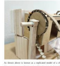
As shown above is known as a replicated model of a chain drive system or mechanism. Just like the actual chain drive system, it functions as a power transmission system to move things power from one place to another. As it is commonly used to transfer power to the wheels of a vehicle, it is also particularly used in bicycles as well as motorcycles. Therefore, it is more utilized in a wide range of machines that require some form of mechanical movement. For a chain drive system to work, there are three separate components that would complement each other to ensure smooth transmission of an object which are the chain, driver sprocket, and driven sprocket. Other than that, properties such as chain length, gear diameter, angle of structure and type of terrain would influence smoothness as well as speed of transmission.
