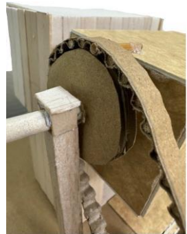
Chain length is crucial as it depends on tension of the mechanism, supplementing the degree of flexibility as well as adaptability. For instance, a shorter chain yields better friction and produces more energy through the responsiveness of the chain and gear. However, range of motion might be limited as it is more rigid compared to a longer chain. Responsiveness depends on gear diameter as it plays a vital role in defining the relationship of torque and speed. Similarly, a smaller gear would generate less torque, which sustaining heavier load becomes harder even with faster rotational speed.
