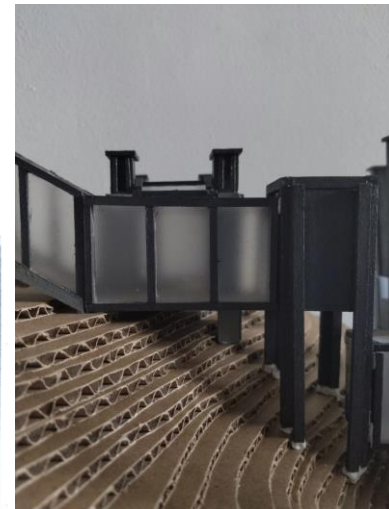
DOUBLE ROW MECHANISM this row can be powered manually by installing pedals in the middle or it can be powered automatically by connecting a pulley with a motor in the middle
