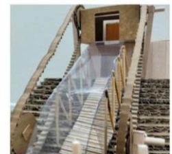
Chain length is crucial as it depends on tension of the mechanism, supplementing the degree of flexibility as well as adaptability. For instance, a shorter chain yields better friction and produces more energy through the responsiveness of the chain and gear. However, range of motion might be limited as it is more rigid compared to a longer chain. Responsiveness depends on gear diameter as it plays a vital role in defining the relationship of torque and speed. Similarly, a smaller gear would generate less torque, which sustaining heavier load becomes harder even with faster rotational speed.
