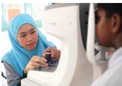
UCSI Student Optometry Association President, Norfaten Anisa Izat uses the auto-refractor to gauge a child's refractive error.
