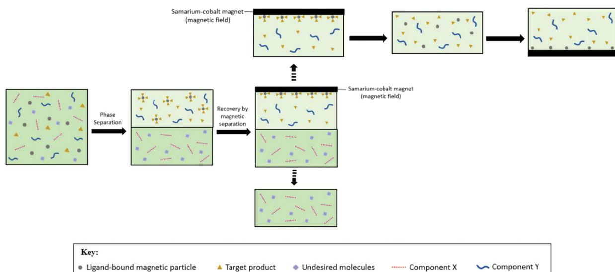
**Figure 2.** Schematic diagram of magnetic ABS.
