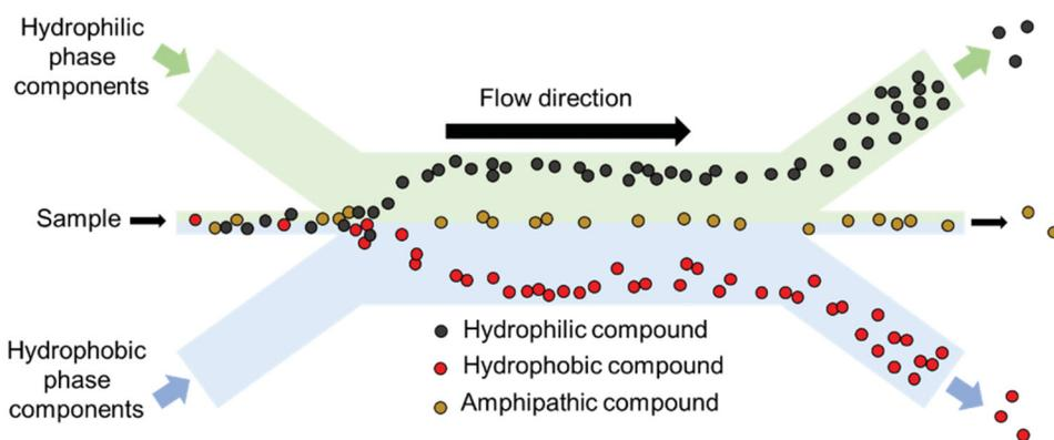
**Figure 4.** Schematic diagram of microfluidic ABS.
