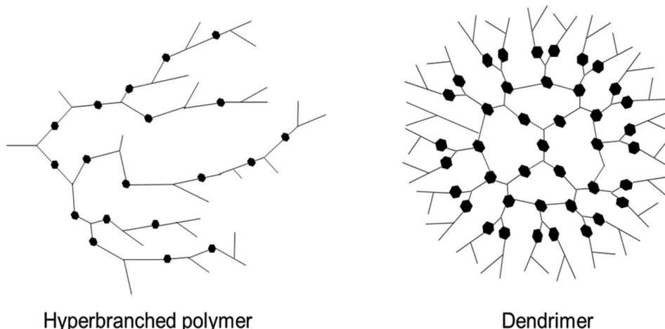
Figure 1. Structures of hyperbranched polymer and dendrimer.
