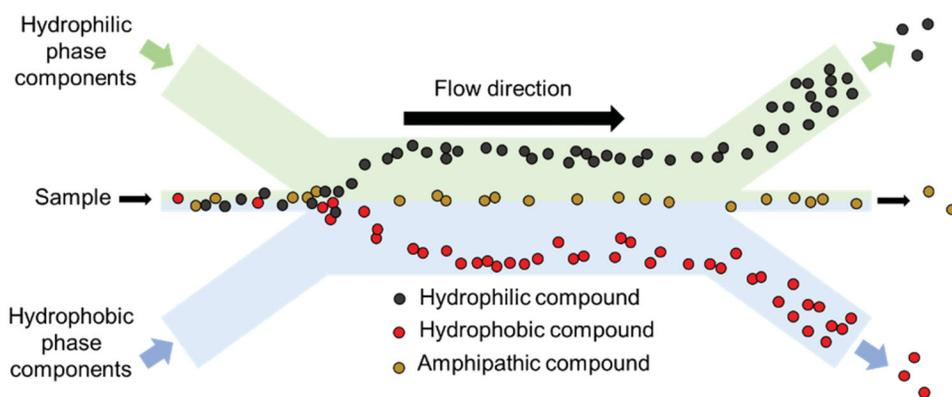
**Figure 4.** Schematic diagram of microfluidic ABS.
