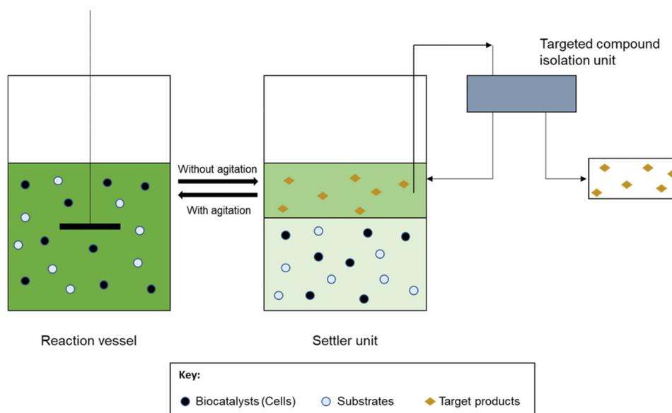
**Figure 6.** Schematic diagram of extractive fermentation and extractive bioconversion using ABS.
