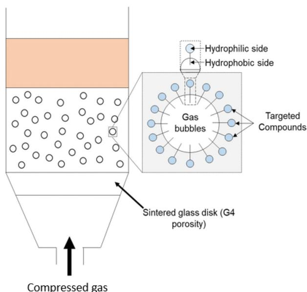
**Figure 3.** Schematic diagram of aqueous biphasic flotation.
